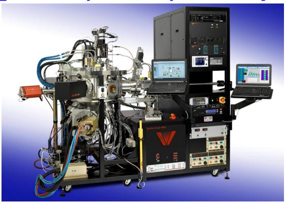
Photograph of a loadlocked magnetron sputter system for 4" diameter wafers. The system includes three 3-inch magnetrons with in-situ tilt, RF biased substrate heater for temperatures of 850°C, and base pressure below 5 x 10<sup>-9</sup> Torr along with an RGA, an UHV three pocket ebeam evaporator, RHEED, and Ellipsometry.
