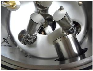
Three UHV Magnetrons with Insitu Tilt, Chimney's and shutters along with QCM & RHEED
