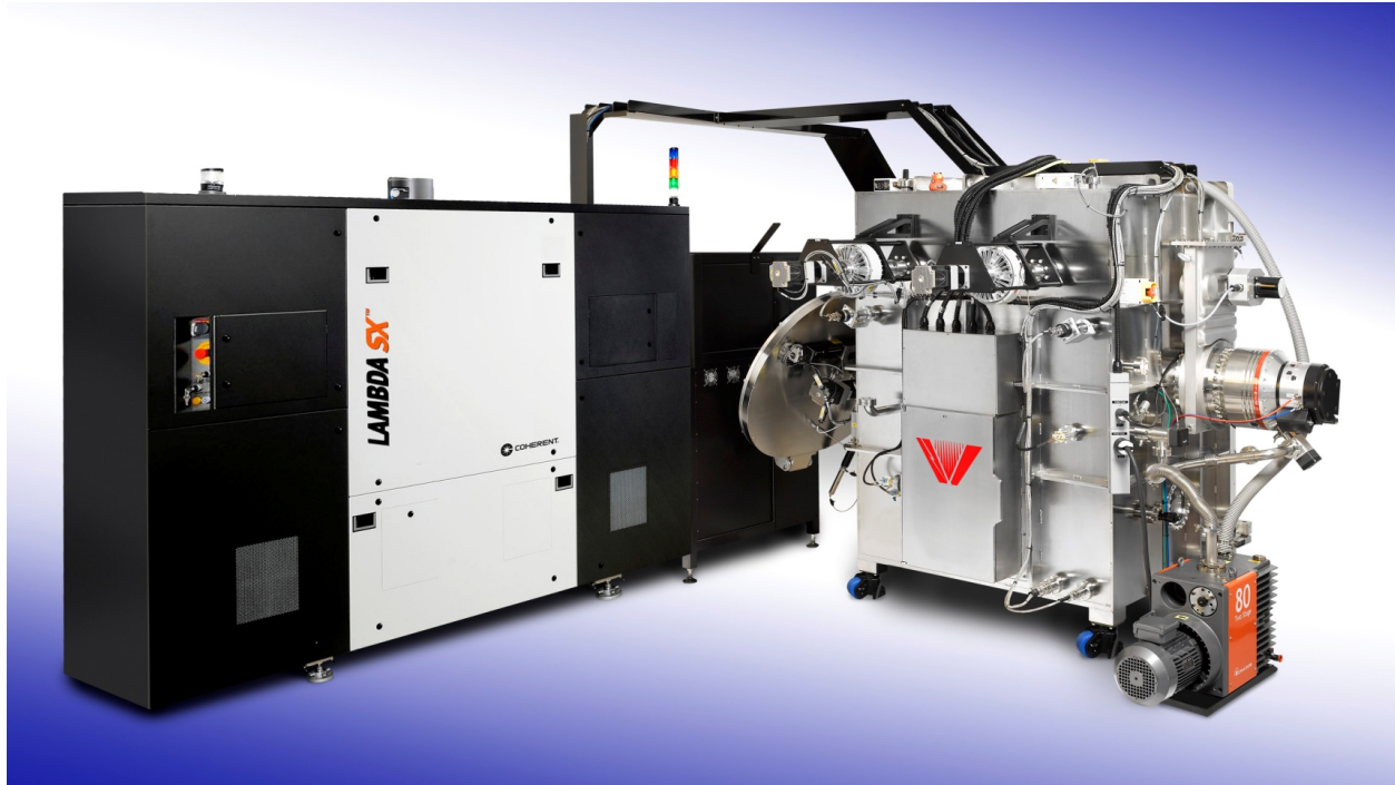
Rear View of a Gen II PLD tool with Coherent 300 Watt Excimer Laser
