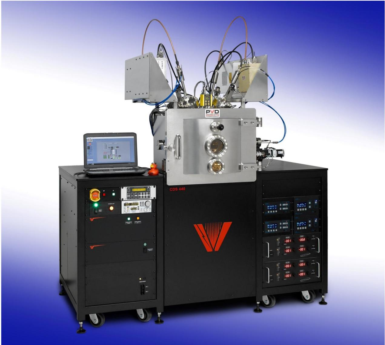
**A sputtering system for growing multiple combinatorial thin film test pads on substrates up to 100 mm in diameter. The system includes four magnetrons with four DC power supplies, two RF power supplies along with a programmable X-Y Stage and mask assembly. The system is an ideal way to create combinatorial libraries of new material compositions in a quick and reproducible fashion.**
