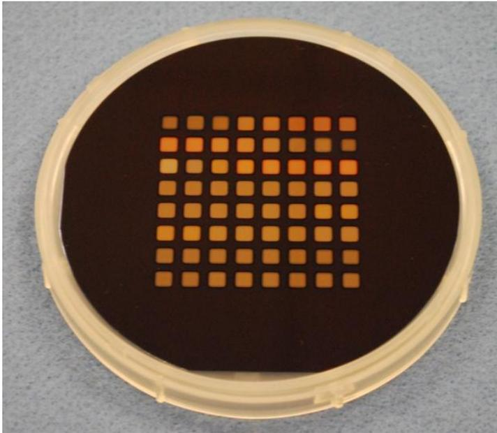
Photograph of a 100 mm diameter Si wafer with an array of 64 different test pads 4 mm square each with a different composition. Compositions can be binary, ternary, or quaternary depending on your need and system design. Concentrations of elements can vary from less than 1 to over 99% depending on deposition conditions. In the case shown the materials used were Cu, Ti, V, and Al. Oxides, carbides, etc can also be fabricated as required.
