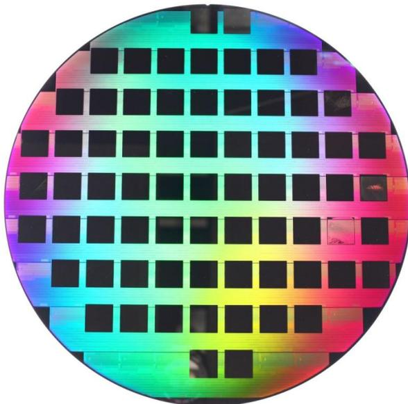
**Photograph of a 300 mm diameter wafer with 68 test pads deposited over pre-patterned underlying circuits for quick electrical evaluation of each test pad composition's electrical properties. After deposition of each test pad it was then capped with a metallic layer to form the final device for electrical testing purposes.**
