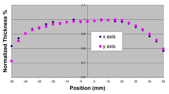
Film Thickness obtained from depositing a 100-nm thick film with a 2-inch Titan Magnetron using a Cu target. The film was deposited at 300 Watts DC onto an oxidized *non-rotating* Si wafer in 5 mTorr (Ar), using a target-to-substrate distance of 4-inches. Measurements were made via a 4-point probe in two mutually perpendicular directions (X, Y) across the wafer surface. A uniformity of  $\pm$  5% is obtained over a 3.5" (90 mm) area.
