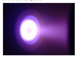
Photograph of a PVD Products 2-inch Titan Magnetron sputter source operating at 100 Watts and 5-mTorr of Argon gas with a Ti target.
