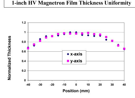
Normalized Film Thickness obtained depositing a ~200-nm thick film with a PVD HV Magnetron with a 1-inch Cu target. The film was deposited onto an oxidized *non-rotating* Si wafer using150 Watts DC in 10 mTorr (Ar), with a target-to-substrate distance of 3-inches (75-mm). Measurements were made via a 4-point probe in two mutually perpendicular directions (X, Y) across the wafer surface.
