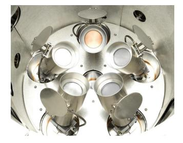
Magnetron Sputter System Interior PVD sputtering system with 5 Titan con-focal magnetrons with tilt & pneumatic shutters
