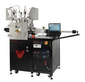
Sputter-Down Box Style Chamber Four 2" Titan Magnetrons, 100 mm RF biased 850°C substrate heater, load lock and full computer control.
