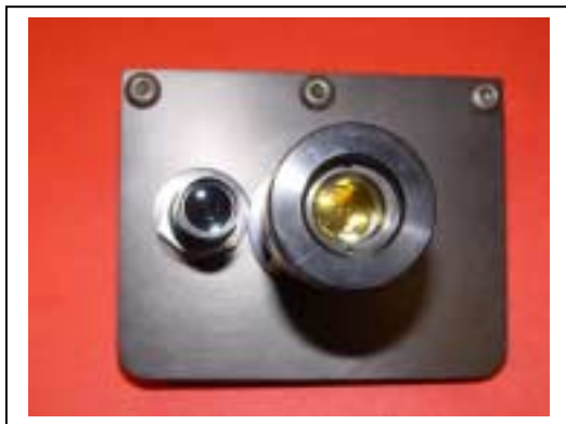
Photo showing the fiber optic beam delivery and pyrometer optical assembly.
