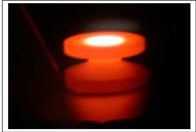
25-mm diam. Inconel Block heated in O 2 to 850°C by a 150-Watt Laser Heater. The bright spot on the top surface has a temperature of 1,200°C.
