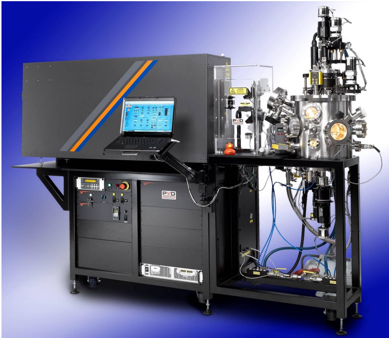
Photograph of a PLD-2000 MBE style deposition system for 2-inch wafers.
