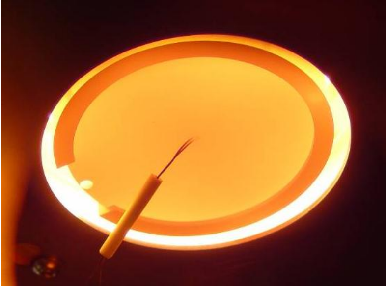
2 inch diameter Inconel disc at 975°C with TC for calibration. Samples just sit in holders – no sliver paste is required.
