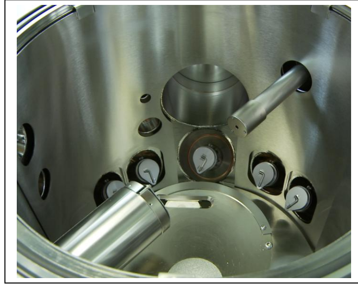
Inside a PLD/MBE 2500 with five effusion cells and Staib HP RHEED gun and re-entrant screen.
