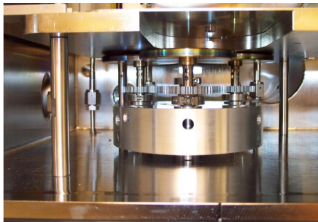
PLD-2000 four position target carousel assembly
