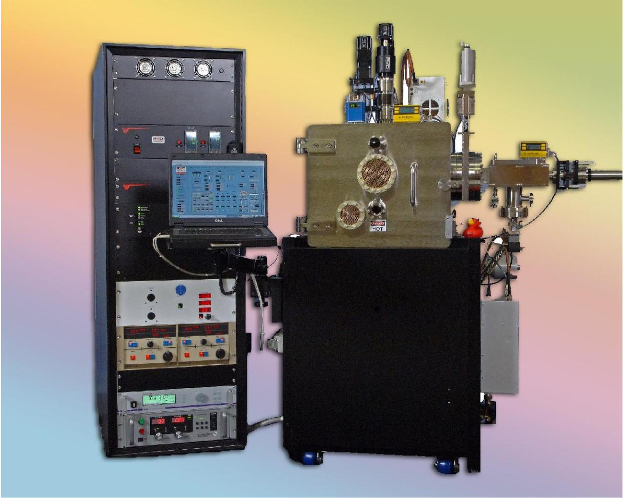
Shown above is a combination three-source magnetron sputtering system with a single thermal evaporation source. Includes an RF biased substrate heater to heat 4-inch substrates to 800°C along with a loadlock for quick substrate transfers. CE marked.
