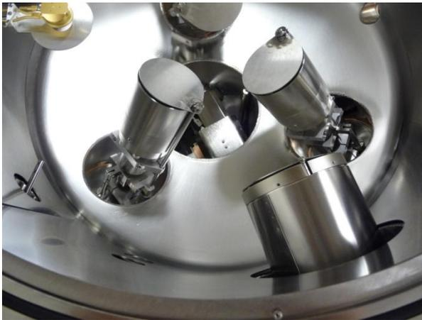
Three UHV Magnetrons with In-situ Tilt, Chimney's and shutters along with QCM & RHEED
