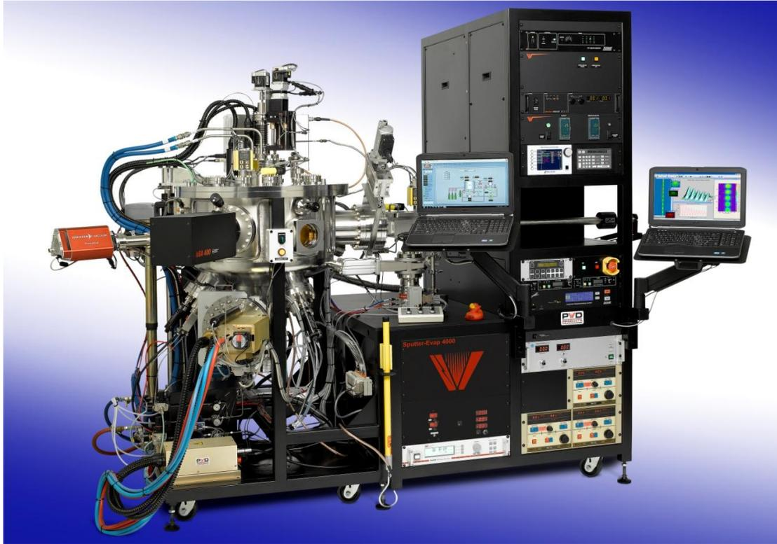
**Photograph of a loadlocked magnetron sputter system for 4" diameter wafers. The system includes three 3-inch magnetrons with in-situ tilt, RF biased substrate heater for temperatures of 850°C, and base pressure below  $5 \times 10^{-9}$  Torr along with an RGA, an UHV three pocket ebeam evaporator, RHEED, and Ellipsometry.**
