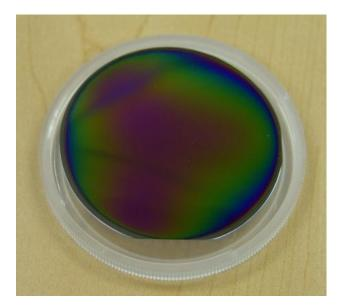
Photograph of a 50 mm diameter wafer with three materials deposited via PLD providing a continual compositional spread across the wafer surface. This is another approach to combinatorial deposition. Please contact PVD Products for more information.
