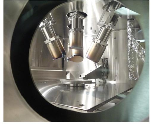
Photograph of the inside of a 300 mm diameter Combinatorial Sputter system showing four magnetrons and a metal mask on a programmable vacuum compatible stage. Each magnetron is also mounted on a computer controlled Z-stage to adjust target-to-substrate distance for fine adjustment of deposition rates.
