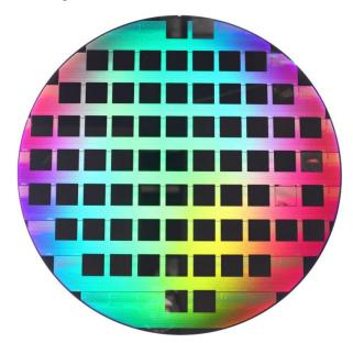
Photograph of 300 а mm diameter wafer with 68 test pads deposited over prepatterned underlying circuits for quick electrical evaluation of each test pad composition's properties. electrical After deposition of each test pad it was then capped with a metallic layer to form the final device for electrical testing purposes.
