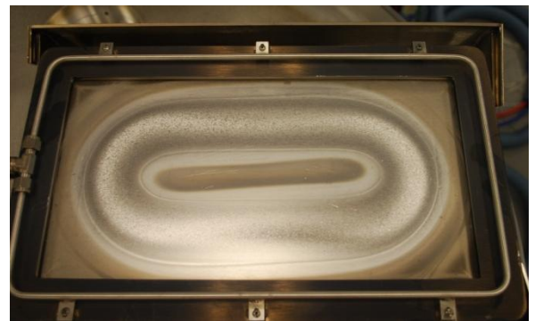
Linear Magnetron with Metal Target and gas injection ring
