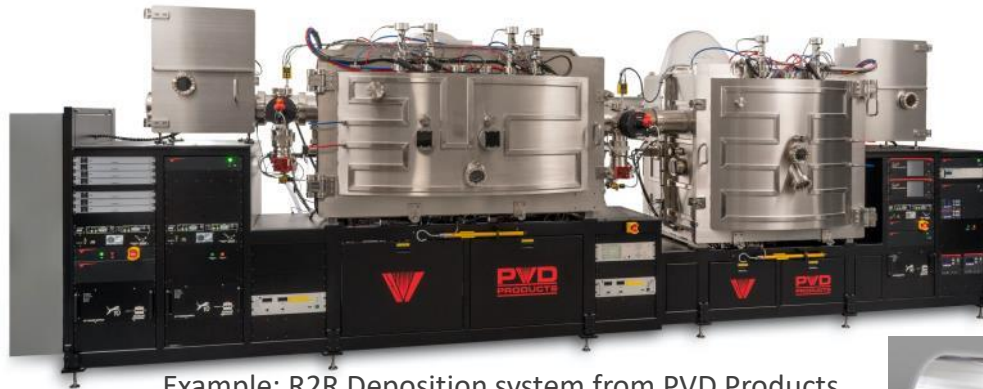
Example: R2R Deposition system from PVD Products
