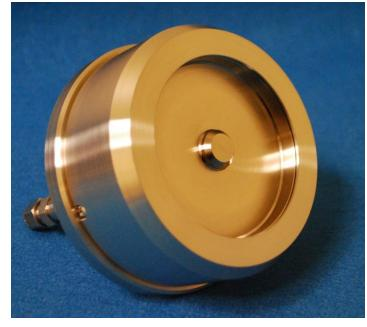
• The bottom flange is a Conflat at ground potential, allowing the head to be mounted on a re-entrant nipple or Z-stage, for setting the desired target-to-substrate distance.
